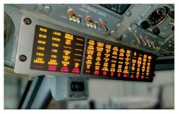
Bright, laser crisp indicia combined with unparalleled off-angle viewing assures both the panels and matching switches are easily read by either pilot. Legends which were previously scalding hot and illegible are replaced with bright modern-day LED technology for better decision making and improved situational awareness.
